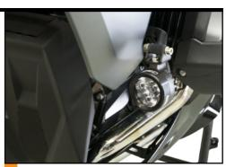
After Light Mounts are secure, re-mount lights using existing hardware. Be sure to postion the lights correctly and check before riding.
