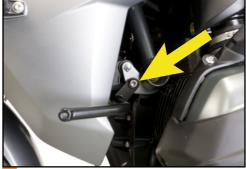
2 Use T40 Torx Driver and 13mm wrench to remove stock mounting bolts.
