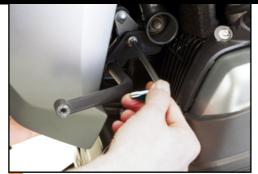
5 Position each Light Mount as shown and and secure using supplied hardware.
