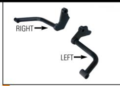
4 To mount MaMo Light Kit, first determine correct orientation of parts. The left side Light Mount, must be fitted to left side of the bike and vice versa.
