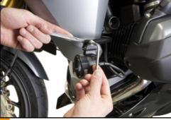
Disconnect lights from stock mounting bracket using 5mm allen wrench and 10mm wrench. Hanging wire can be used to secure lights while mounts are replaced.
