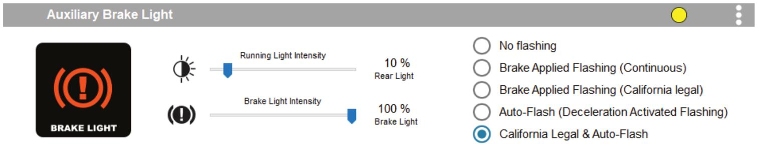
The Auxiliary Brake Light settings interface includes a 'BRAKE LIGHT' icon and two sliders: 'Running Light Intensity' set to 10% Rear Light and 'Brake Light Intensity' set to 100% Brake Light. On the right, there are five radio button options: 'No flashing', 'Brake Applied Flashing (Continuous)', 'Brake Applied Flashing (California legal)', 'Auto-Flash (Deceleration Activated Flashing)', and 'California Legal & Auto-Flash' (selected).
