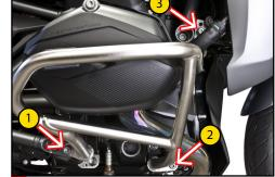
To mount AvantGuard Light Bars with OEM crash bars, loosen bottom two mounting screws (1 & 2) and remove top screw (3) entirely. (RIGHT SIDE SHOWN)
