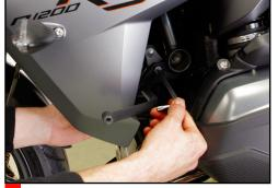
Position a Light Bar against the frame mounting flange. Insert an M8 screw with washer & secure with a washer and nut behind the frame flange. (LEFT SIDE SHOWN)
