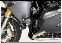
After Light Bars are secure, mount lights using existing hardware. Be sure to align the lights correctly and re-check tightness.
