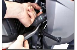
2 Carefully align crash bar mounting hole with Light Bar mounting hole so that the screw can be started by hand to avoid cross-threading. Screw into welded nut on crash bar flange.
