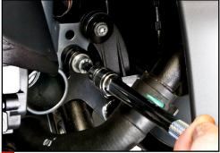
Once light bar is in position, tighten all crash bar mounting screws. Mount light fixture as shown above.
