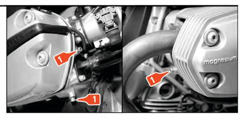
Position an X-Head over the cylinder head, aligning the mounting holes with the bosses on the engine.
